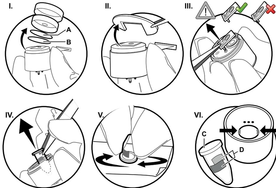
During calibration of the PID, the gas detector recognises a dirty lamp and triggers a corresponding warning. If this warning is displayed, the lamp window must be cleaned. To clean the lamp window, silicon-free single-use gloves and the DrägerSensor PID cleaning set (order number 83 19 111) must be used. The cleaning set can only be used once.
