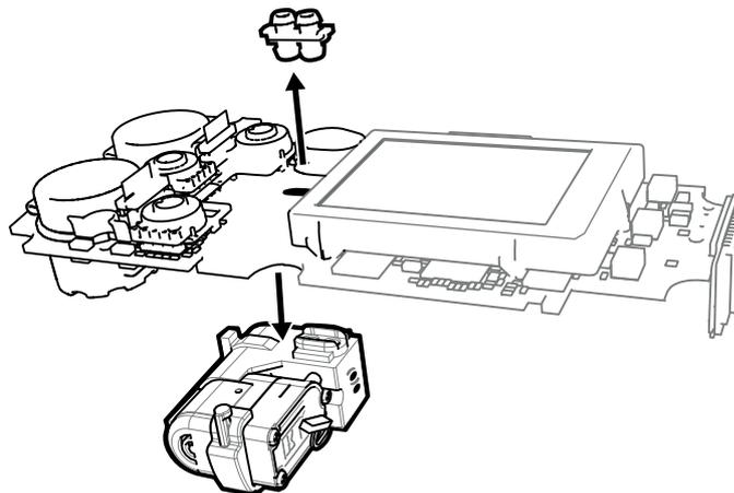
9. Pull pump out of pump block.
