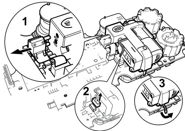
5. Carefully remove the flexstrip with the differential pressure sensor (1) from the pump block.
